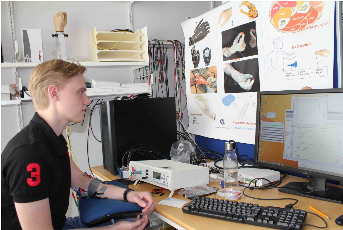
Figure 7.7: The subject doing the test. The subject looks at the screen to see the commanded motions and gets visual feedback from the bars.
