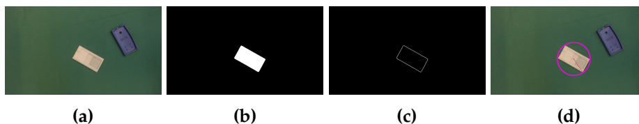
Figure 9.6: (a) The original RGB image, (b) the corresponding binary image of a white cover, (c) drawn contours of the BLOB and (d) the minimum enclosing center, center of the BLOB and radius.
